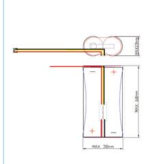
Thickness: 19mm Width: 38mm Height: 69mm
