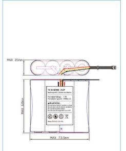
Thickness: 20mm Width: 73.5mm Height: 68mm
