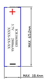
**Diameter: 18.4mm Height: 65.2mm** (Note:Drawings just for reference)
